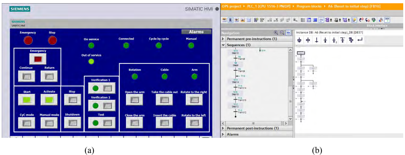
Figure 6.45: The reset to initial state mode (A6) of GEMMA is off, while the reset process has been finished. (a) the screen, (b) the program
