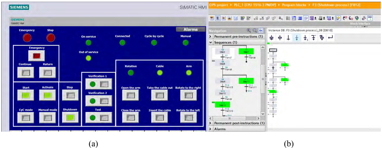
Figure 6.37: The program is placed at the shutdown process mode (F3) of GEMMA, while the shutdown process is operated, arm is closing. (a) the screen, (b) the program
